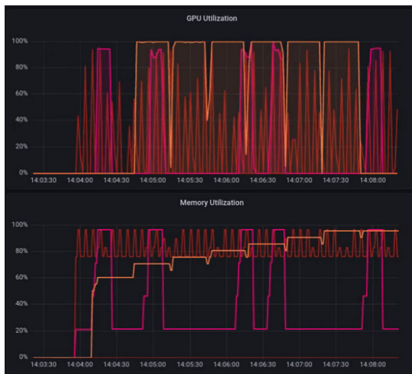
Figure 5. Monitoring a MIG partitioned GPU per instance
